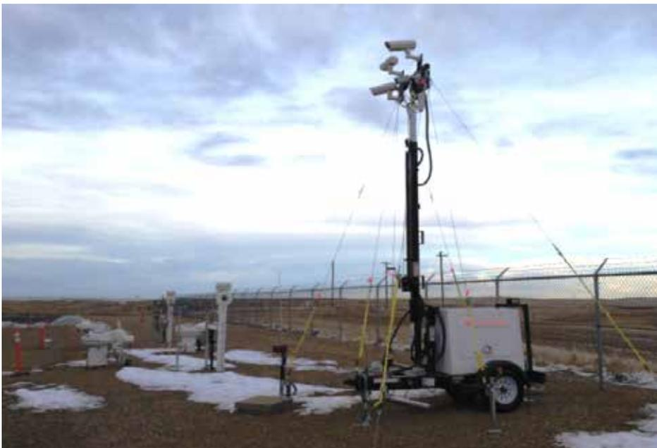
An IntelliView trailer in the field: The weatherproof and self-contained trailer can accommodate multiple DCAM™ units and green power options (fuel cell and solar panels). The DCAM offers an effective way of detecting and alerting on small above-ground fluid spills, sprays, and pooling within seconds.
